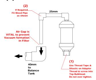
NOTE: It is vital that the connection to the balance tank includes an "Air Break" as shown above to prevent a vacuum being formed within the filter. This "Air Break" should be positioned as close as possible to the Kinetic Valve.
