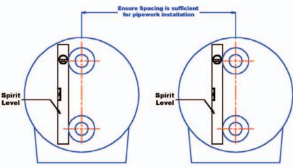
NOTE: Do not fill with filter media until face plumbing & drain valve have been installed
